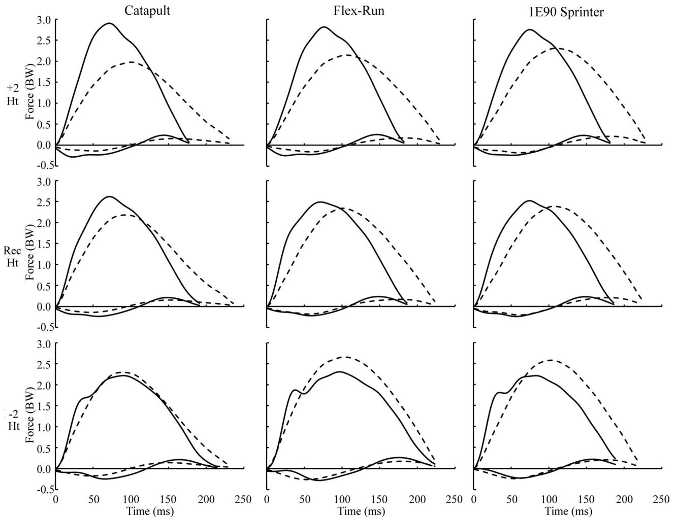
Fig. 7. Mean vertical and horizontal GRFs from 10 consecutive affected (broken line) and unaffected (solid line) leg steps from a representative participant running at 3 m/s. Columns *left to right* indicate the Freedom Innovations Catapult FX6, Össur Flex-Run, and Ottobock 1E90 Sprinter prostheses. Rows *top to bottom* indicate prosthetic height: +2 cm, recommended (Rec), and -2 cm.
