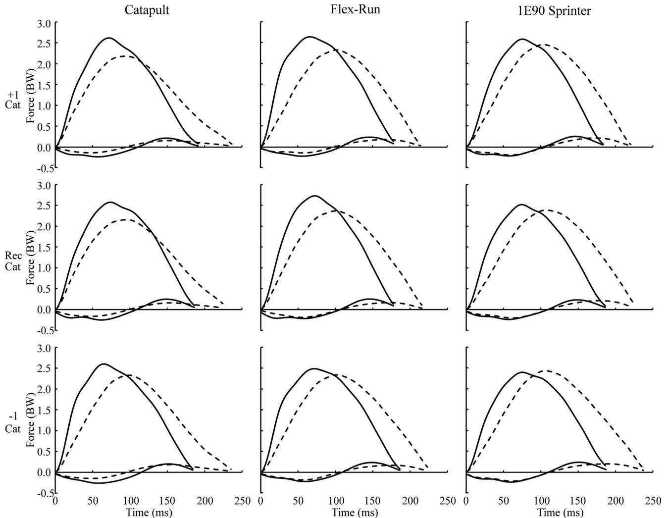
Fig. 6. Mean vertical and horizontal GRFs from 10 consecutive affected (broken line) and unaffected (solid line) leg steps from a representative participant running at 3 m/s. Columns *left to right* indicate the Freedom Innovations Catapult FX6, Össur Flex-Run, and Ottobock 1E90 Sprinter prostheses. Rows *top to bottom* indicate prosthetic stiffness category: -1, recommended (Rec), and +1.
