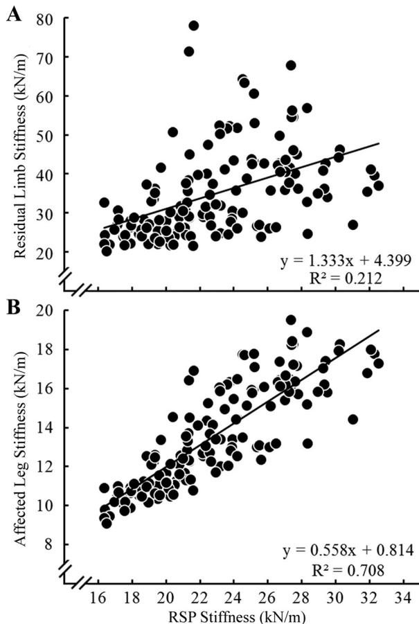
Fig. 4. A: residual limb stiffness compared with running-specific prosthetic (RSP) stiffness ( $P < 0.001$ ). B: affected leg stiffness compared with prosthetic stiffness. We performed linear regressions across all collected data to determine significant correlations between residual limb stiffness and RSP stiffness ( $P < 0.001$ ) (A) and between affected leg stiffness and RSP stiffness ( $P < 0.001$ ) (B).
