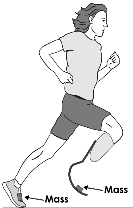
Fig. 1 The center of the added mass was adhered 10 cm from the distal end of the shoe on the unaffected leg and of the RSP on the affected leg
